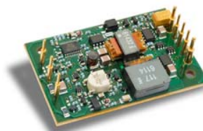
Figure 2 PKM-E 1/4-brick 25A/82.5W Size LxWxH 57.9x36.8x8.5 (12.7)mm
